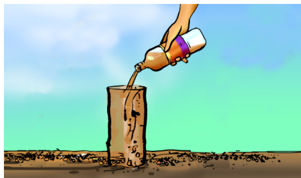
Fig. 9.5 Measuring rate of percolation
