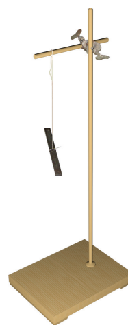
Fig. 13.9 A freely suspended bar magnet always comes to rest in the same direction
