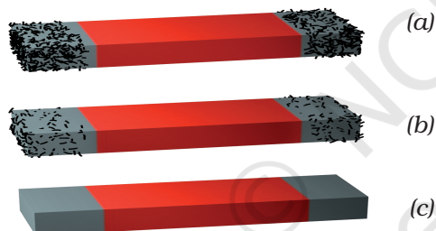
Fig. 13.6 Magnet with (a) many iron filings (b) few iron filings and (c) no iron filings sticking to it.
